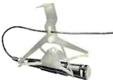
ALTEC 689A CARDIOID DYNAMIC MICROPHONE —$108 net. High front-to-back discrimination for an average of over 20 db from 40 to over 16,000 cycles. Virtually flat response throughout this frequency range. Output Impedance: 30/50, 150/250 and 20,000 ohms (selection by connections in microphone cable plug). Output Level: -54 dbm/10 dynes/cm 2 . Hum: -120 db (Ref.: 10 -3 Gauss). Dimensions: 1 1/4" diameter at top, 7 1/4" long not including plug. Weight: 11 ozs. (not including cable and plug).
